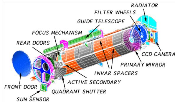
Figure 9: Cutaway figure of the *TRACE* instrument
