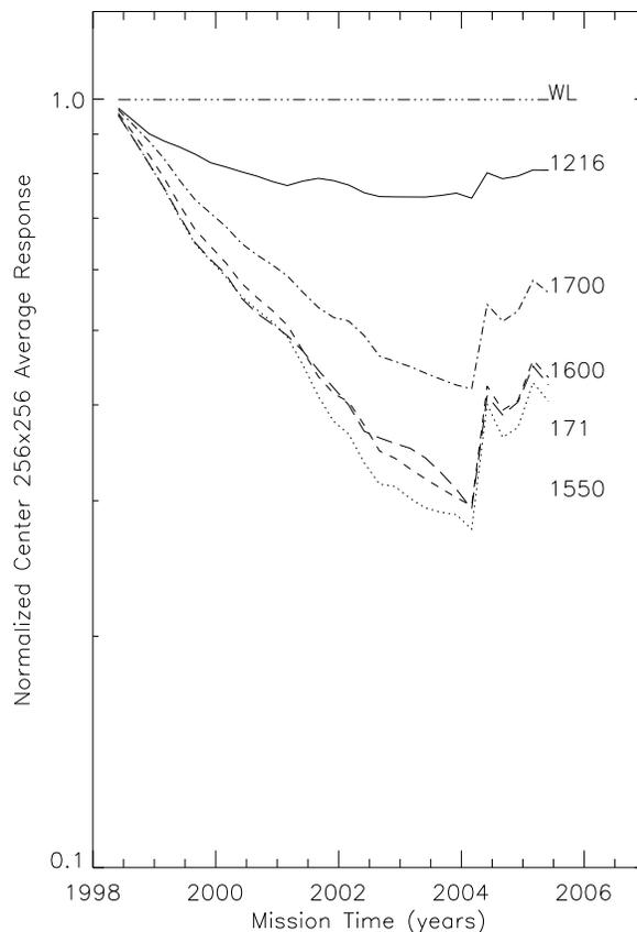
Figure 11: *Relative responses of the TRACE band-passes at the center of the field of view. Several CCD annealings have rejuvenated the detector sensitivity to a level equivalent to early in 2001.*
