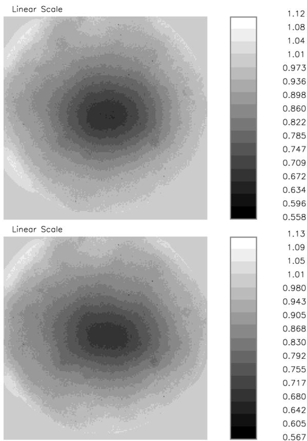
Figure 10: The top image shows the 1700 Å flat fields (relative response) for 6 June 2005. This current flat field, after repeated CCD annealings, is very similar to the lower one for 1 May 2002 because of the increase in sensitivity caused by repeated CCD annealing. Flat fields for other wavelengths are qualitatively similar.
